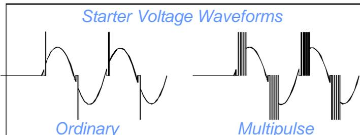
Under normal conditions a lamp will strike, after heating, on the first pulse received and further pulses are inhibited - so the Multipulse starter provides a positive soft start typical of a single pulse starter. The Multipulse advantage becomes evident under limit conditions of low ambient temperature and low supply voltage.
